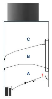
Flue gas opening 1 can be adjusted using adjustable smoke deflection plate A. The setting depends on the chimney's natural draw and affects the combustion and efficiency of the fireplace. By default, the opening is set to maximum efficiency.
