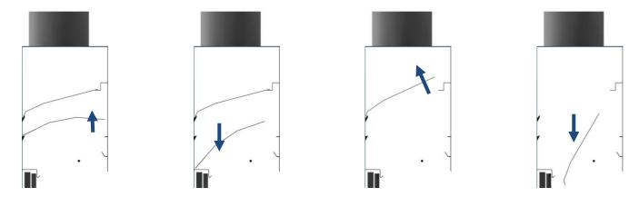
The plates need to be removed to facilitate the cleaning of the chimney. Moving the top smoke deflection plate is done in exactly the same way as removing the bottom plate (lift it upwards, move it forwards, move the back downwards: see the bottom of the previous page).
